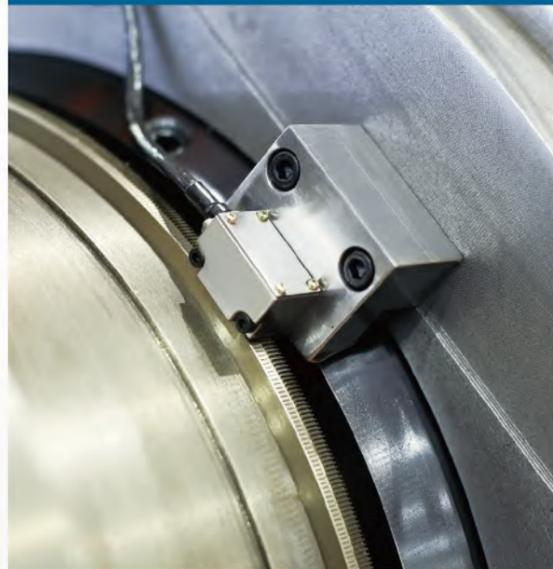
The LA series with C-axis positioning allows driven tool milling avoiding artifacts generated by compounding movement errors, giving higher accuracy with shorter process times and less effort.
