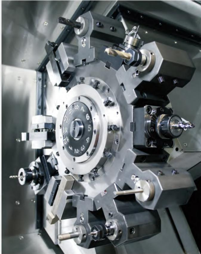
The turret is designed for extreme rigidity through its wide and heavy build, inclusion of heavy duty oversized couplings and enhanced clamping pressure.
