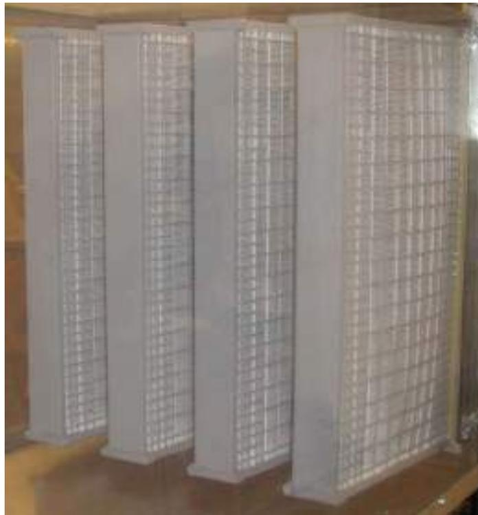
Air filter MV-F7-03-A-S-D-RPG-Y-H23-03 at a differential pressure of about 4000 Pa.
