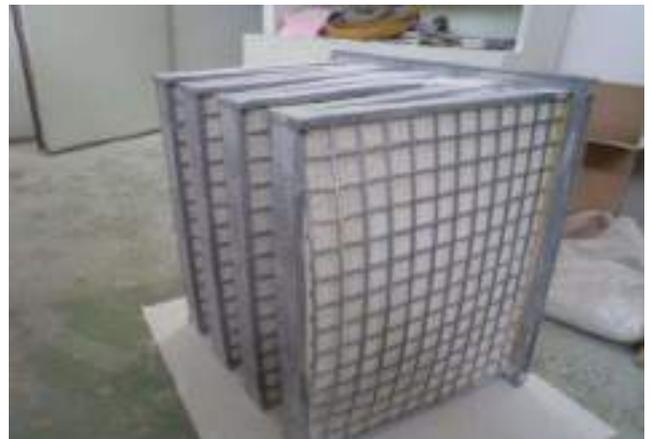
Air filter MVX-E10-03-A-S-D-PG-Y-H23-03 at a differential pressure of 6100 Pa.
