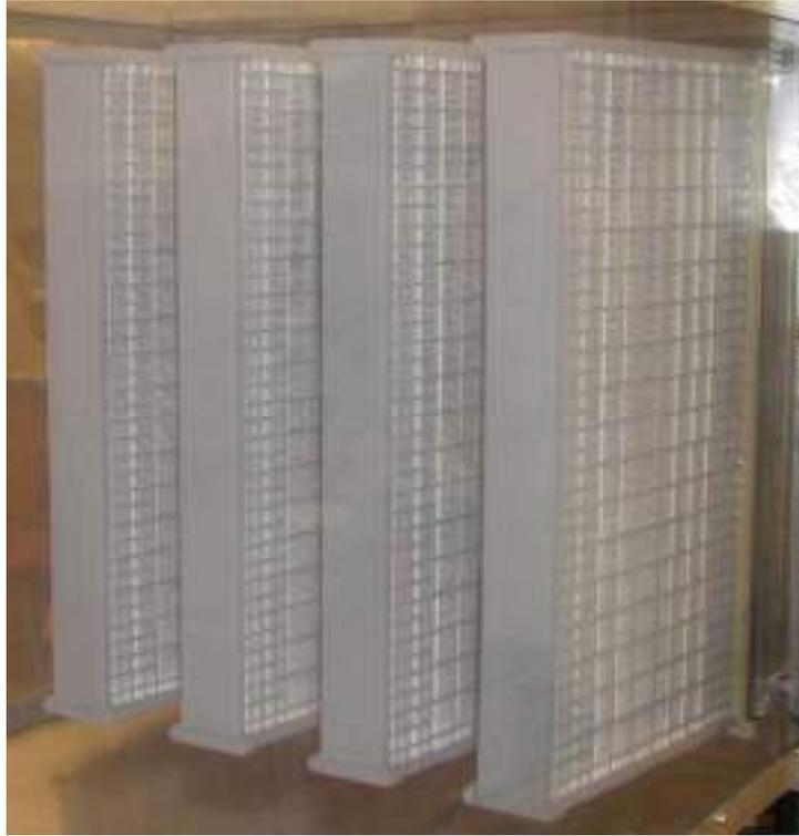
Air filter MV-F7-03-A-S-D-RPG-Y-H23-03 at a differential pressure of about 3000 Pa.
