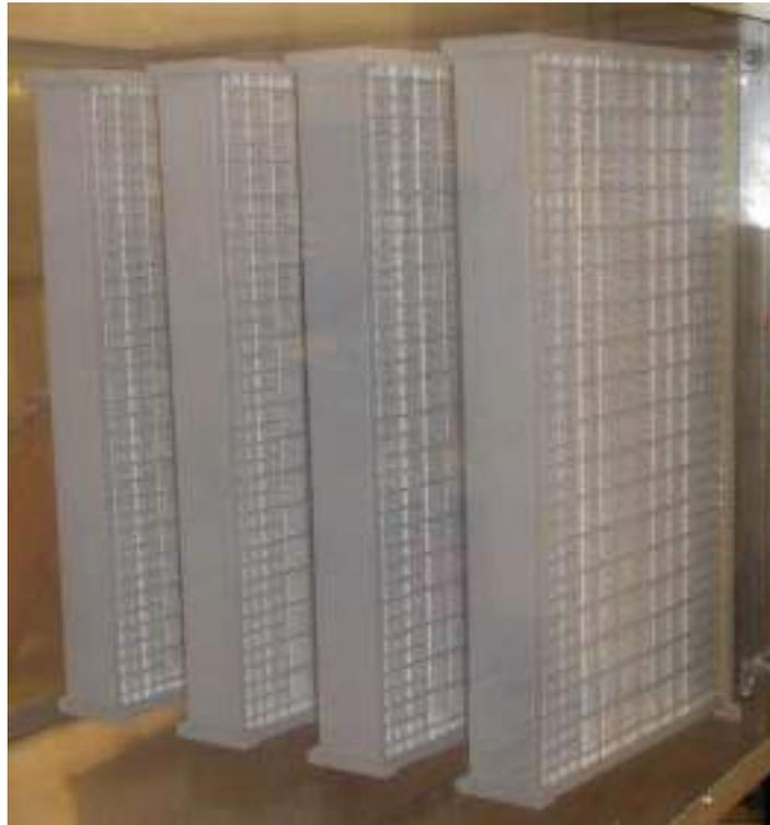
Air filter MV-F7-03-A-S-D-RPG-Y-H23-03 at a differential pressure of about 1500 Pa.
